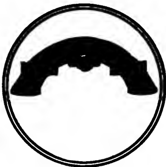
Intake manifold in a jacket of water at outlet temperature. Gas kept at a constant temperature that insures quick vaporizing.
